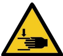
Figure 2: Safety notice "Caution: Crush hazard"
