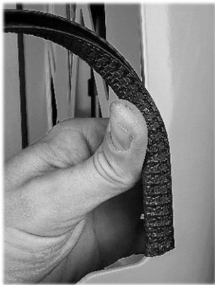
Figure 12: Replacing the edge protector
